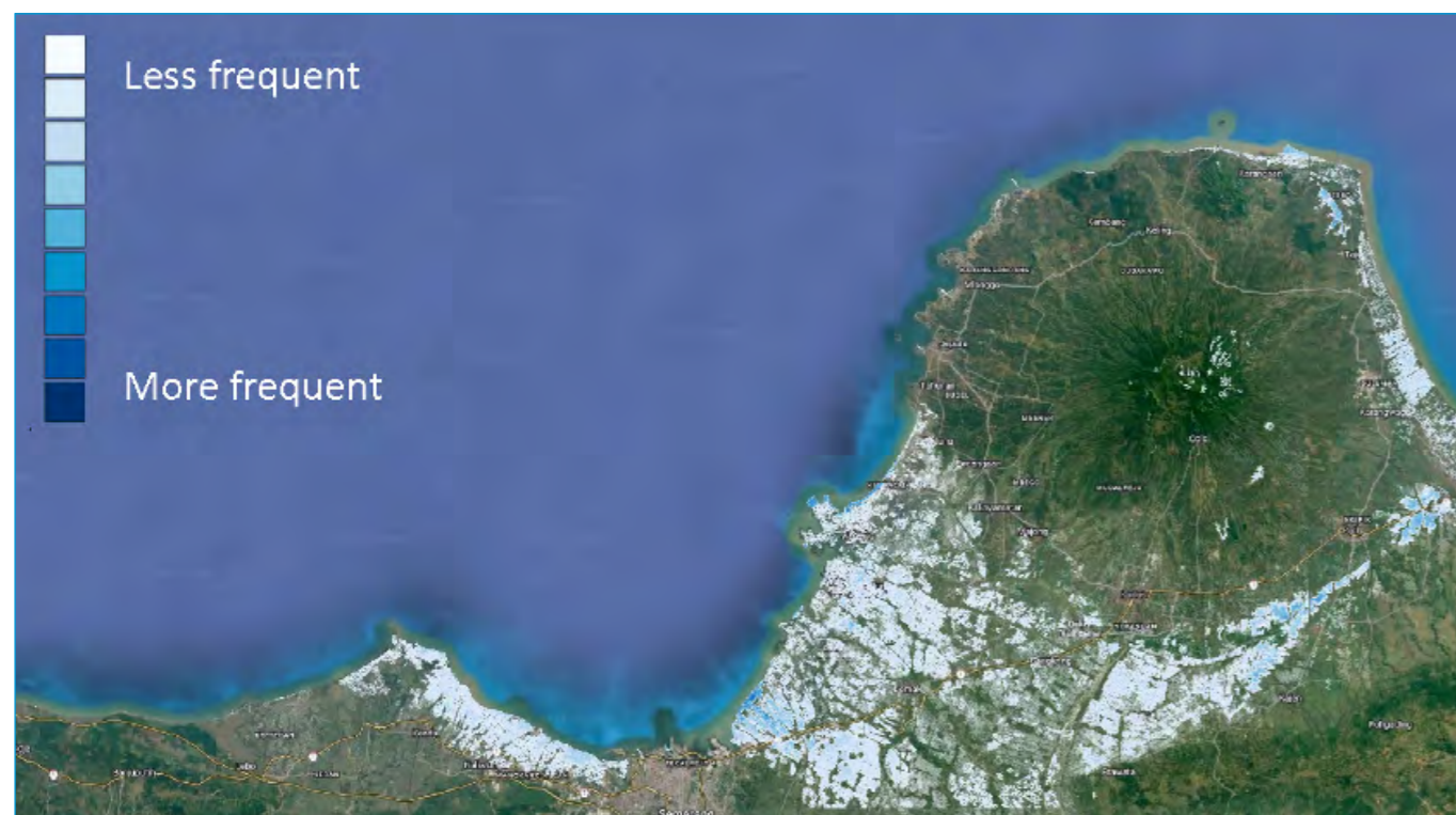
Figure 18. Flood frequency in Surabaya (Indonesia) darker colours depict areas that have been flooded more frequently in the monitoring period here from 2015 to 2023, processed by LIST/CIMA/Wasdi Sari).
